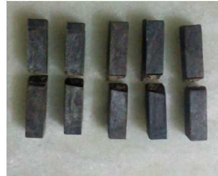
Fig 3 sample specimen after impact test
