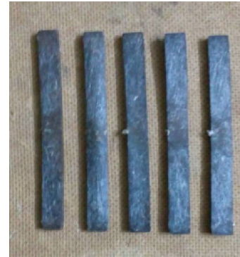
Fig.2 Sample Specimens of Flexural test
