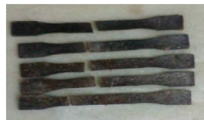
Fig.1 Sample Specimens after Tensile test
